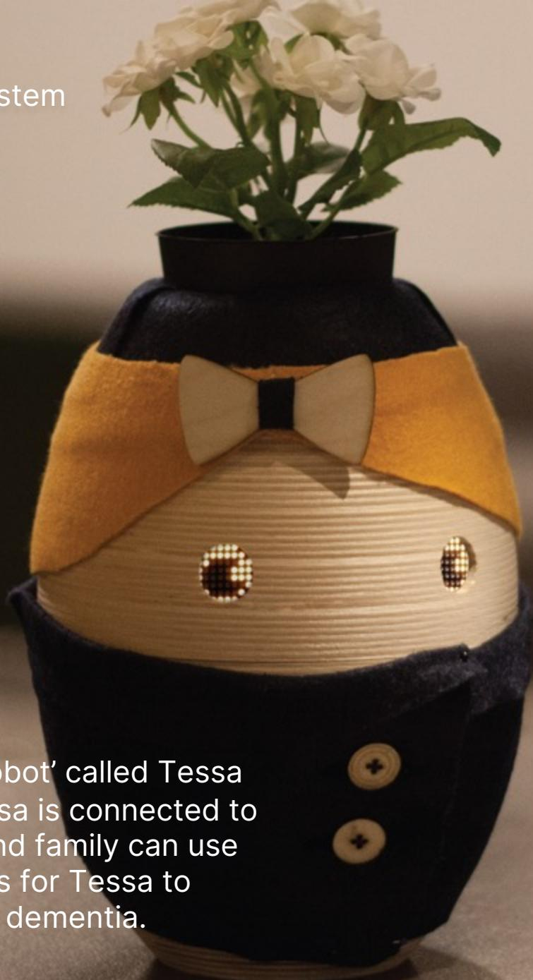
Tinybots has developed a 'social robot' called Tessa that provides verbal guidance. Tessa is connected to the Tinybots system. Caregivers and family can use a web application to schedule tasks for Tessa to provide support to the person with dementia.
